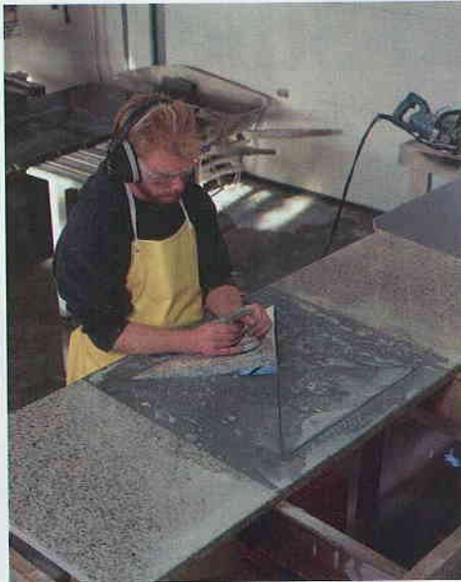
**Easy does it.** Once the cuts have been made, pieces of granite are carefully lifted out of the new openings. The tape is removed from the loose section to allow the suction-cup-based tool to grip the stone.
