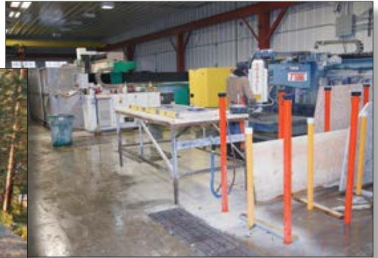
*Above: Seen at right in the foreground, Freshwater Stone's Thibaut T-102 radial arm polisher. At left in the background is a Prussiani CNC, which handles much of the shaping and polishing of the company's slab work.*
